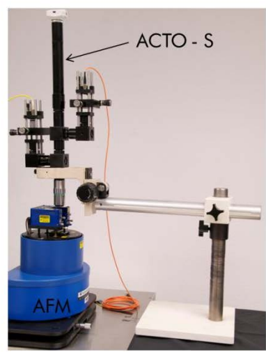
Possible ACTO-S integration with conventional Atomic Force Microscope (AFM)
