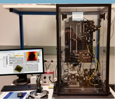
**ACTO-SCM** is a Scanning Laser Confocal Microscope to do:
