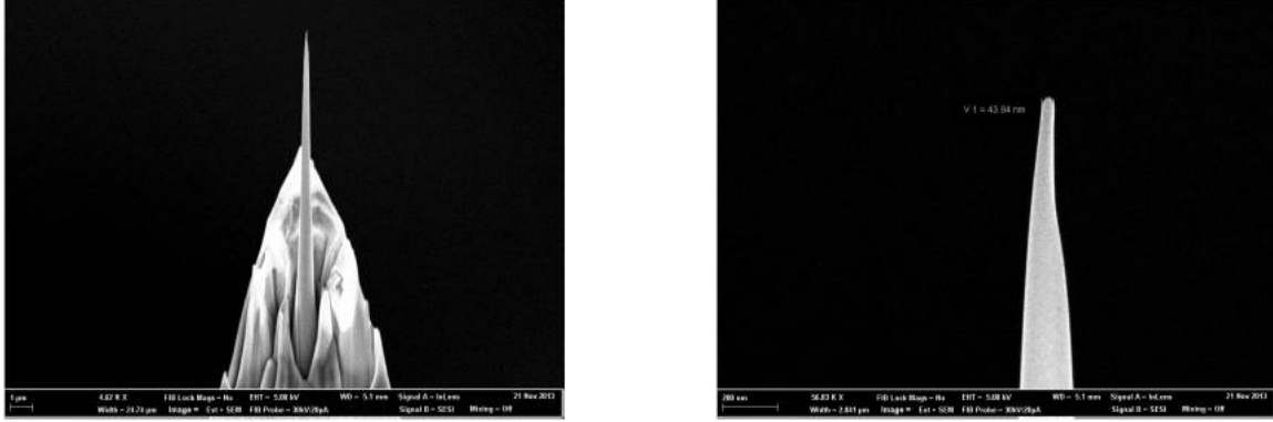
Figure 4. SEM image (left) and enlarged SEM image (right) of high-aspect-ratio probe tips fabricated from TR-400 Olympus probes.
